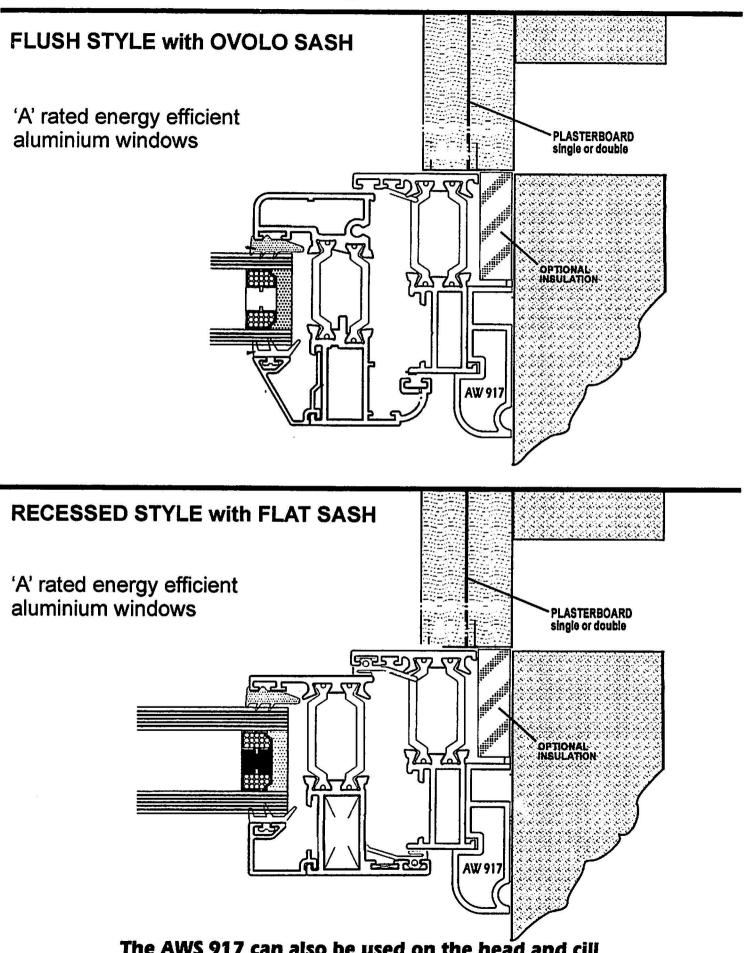
The AWS 917 can also be used on the head and cill or the standard 25mm cill with or without AW 42 head extension
