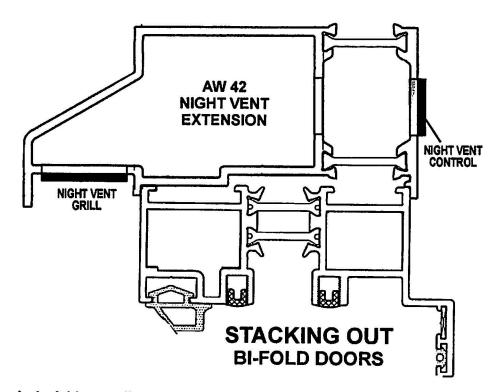
Concealed trickle ventilation with integrated head - no visible external night vents to spoil the appearance of slim aluminium windows and bi-fold doors. Bi-fold doors have a slim frame to frame size of 132mm & high security locking with high performance double glazing (as specified for 'A' rated windows).
